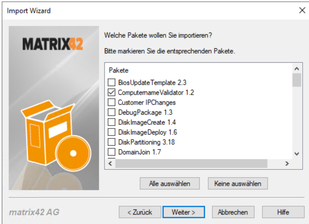
1 – Selection window from the Import Wizard (preferably use 'select none' before proceeding)
